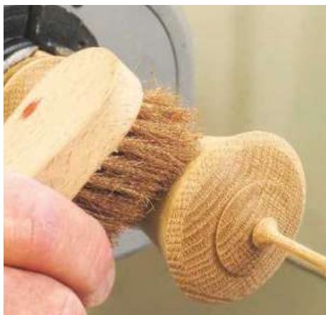
▲ Pic.31 He opted for a lime effect. Use a brass liming brush to clean out the grain. This will not scratch the wood if, wherever possible, you work in the direction of the grain
